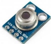
Gambar 4. Sensor Suhu MLX90614 ( https://www.edukasiElektronika.com/2020/09/sensor-suhu-non-contact-mlx90614-gy-906.html )
